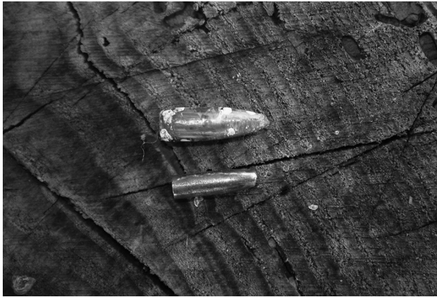
Figure 2.13 Chinese 7.62×39mm projectile and cylindrically shaped mild-steel penetrator. (Image from author's collection.)
